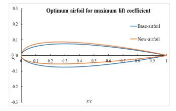
Fig. 3. New airfoil for maximum lift coefficient
