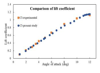
Fig. 2. Validation of lift coefficient at Re=10<sup>6</sup>
