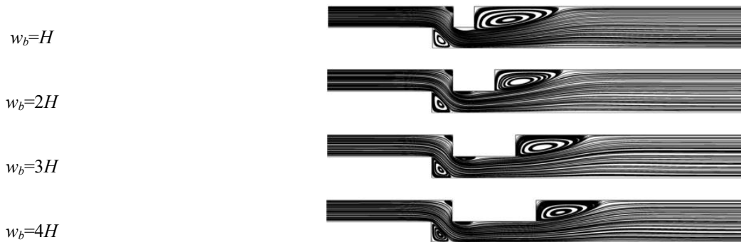
Fig. 2. Streamlines ( \phi=0.03, Re=100, h_b=H ).
