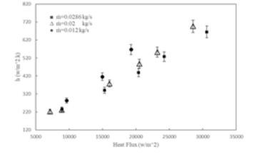
Fig. 3. Variations of heat transfer coefficient at the mass flow rate of 0.02 and 0.0286 kg/s under various heat fluxes in the vertical annulus tube at fixed axial positions of z = 45 cm
