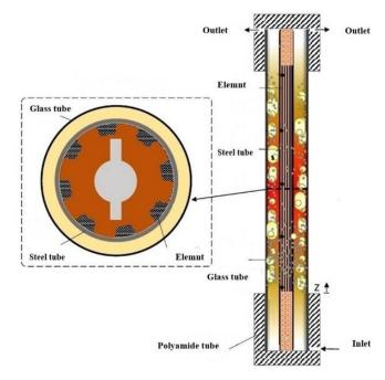
Fig. 2. Schematic design of test section
