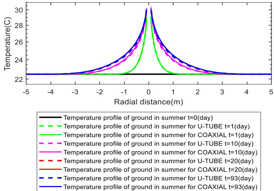
**Fig. 3. Temperature distribution of soil at depth 80 m**
