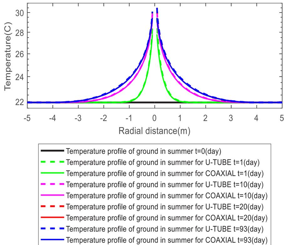
Fig. 2. Temperature distribution of soil at depth 20 m
