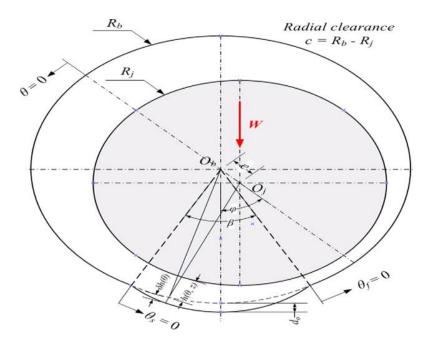
Fig. 1. Journal bearings geometry by considering abrasion
