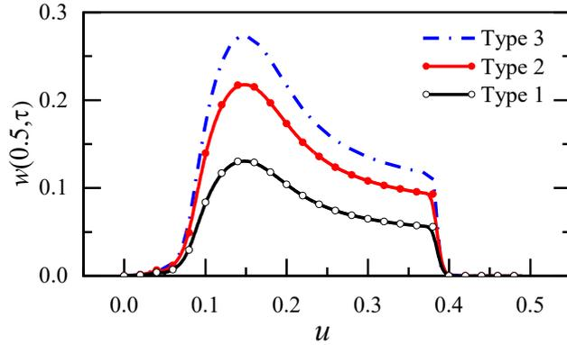
Fig. 2. The maximum amplitude of oscillations of the midpoint of a porous beam in terms of external fluid flow velocity
