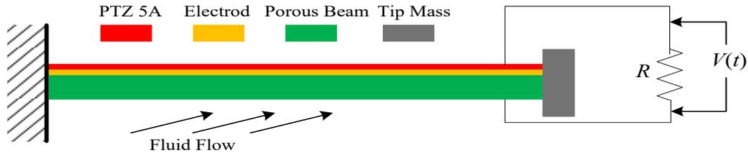
Fig. 1. Configuration of piezoelectric energy harvesting with the core made of porous material
