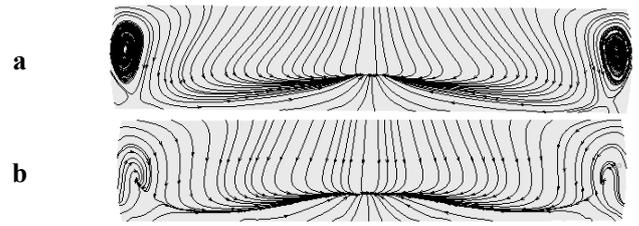
Fig. 2. Secondary streamlines in 80% AS concentric stenosis in the non-planar branch a) Newtonian, b) non-Newtonian
