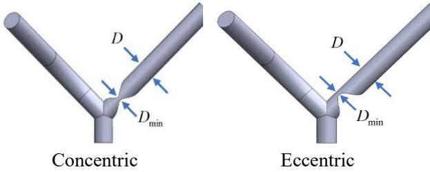
Fig. 1. The geometry concentric and eccentric stenosis
