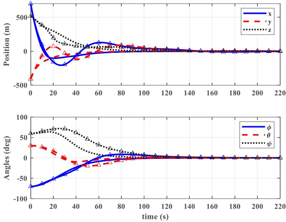
Fig. 1. Time history of the position vector and Euler angles- triangles denote the EKF-PID method results
