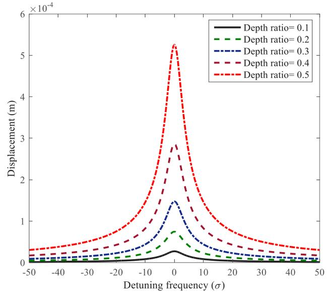
Fig. 6. The effect of crack depth on superharmonic resonance response when  $\Omega = (\omega_0 / 2)$  and  $\eta = 0.9$
