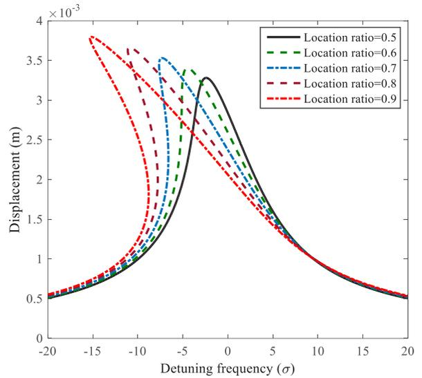
Fig. 4. Frequency-response curves in the primary resonance when location ratio
