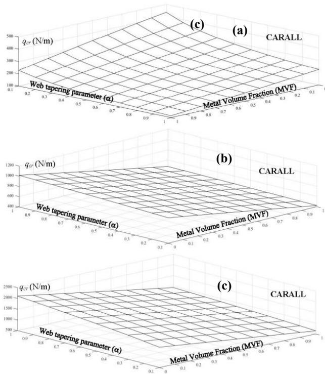
**Fig. 2.** Variation of the lateral buckling load with respect to the metal volume fraction and web tapering for CARALL section for three different transverse loading positions, (a) Top flange, (b) Centroid, (c) Bottom flange
