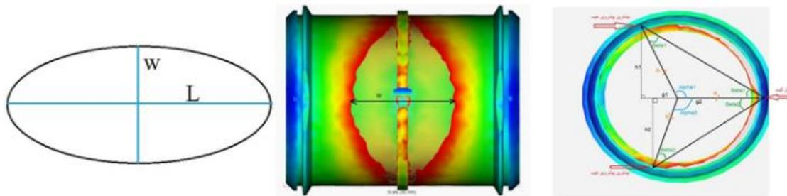
Fig2. Pictures of defect, showing W,L,Alpha1,Alpha2, and R
