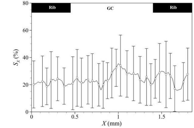
Fig. 2. In-plane saturation profile of liquid water in GDL
