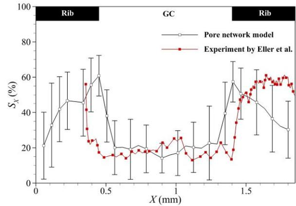
Fig. 3. In-plane saturation profile as a result of the coupled model. The saturation distribution of Eller et al. is also added for comparison [5].
