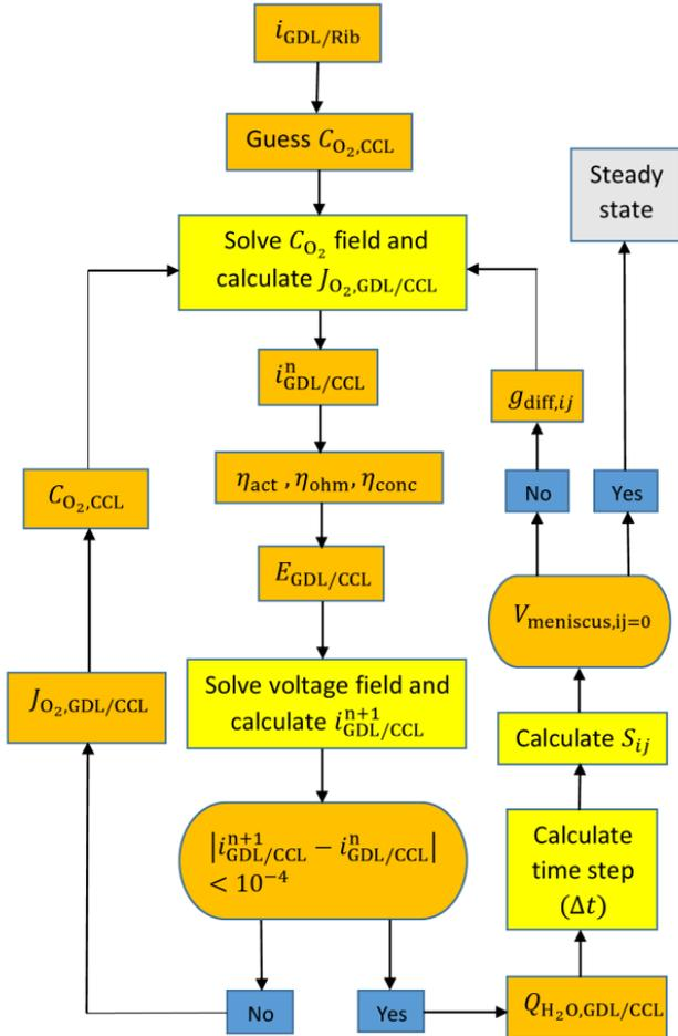
Fig. 1. Coupling algorithm of transport phenomena at the cathode side of the fuel cell
