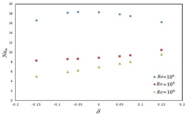
**Fig. 3. Variations of the average Nusselt number of the heat source surface for the flexible system for different values of Ra and  $\delta$**
