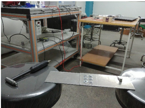
Fig. 3. Configuration of experimental test analysis of single-lap bolt joint
