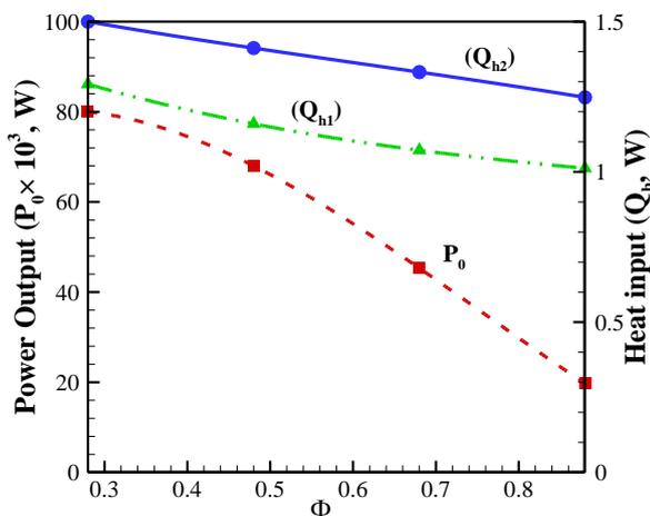
Figure 4. The effect of different cross-sectional area ratio on power output and heat input.
