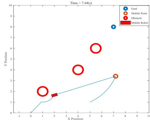
Fig. 4. The path of the robot towards the target and its orientation towards the moving point
