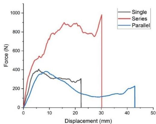
Fig. 1. Force-displacement diagram for egg box cores under compression
