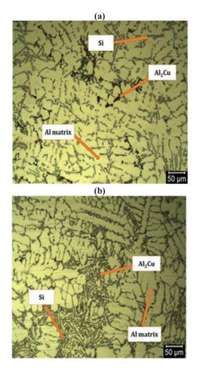
Fig. 1. Aluminum alloy microstructures: (a) without nano-particles and (b) with nano-particles
