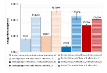
Fig. 2. The effect of the lubricant addition on the FF lifetime of the aluminum alloy
