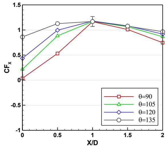
Fig. 3. Comparison of force coefficient in the  $X$  direction at  $\alpha=0^\circ$
