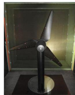
Fig. 1. Image of TU-BERT turbine blade in a wind tunnel
