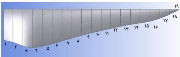
**Fig. 7. Elements of blade**
