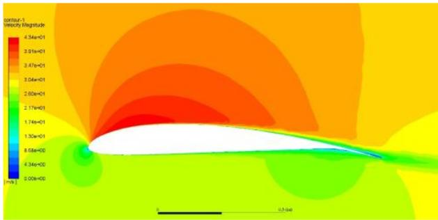
**Fig. 6. Contour velocity around the section at zero degree of attack angle and Reynolds number 200,000 Cross-section with flap 15%**
