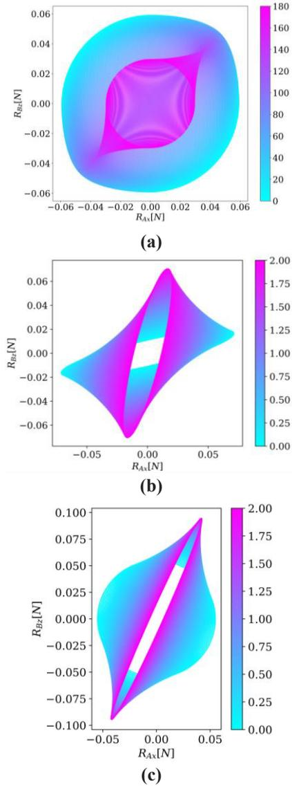
**Fig. 1. sample diagrams of force patterns in symmetrical dynamic unbalance for: (a) angular difference of unbalance particles, (b) unbalance distance from bearings, and (c) distance of unbalance center from bearings**
