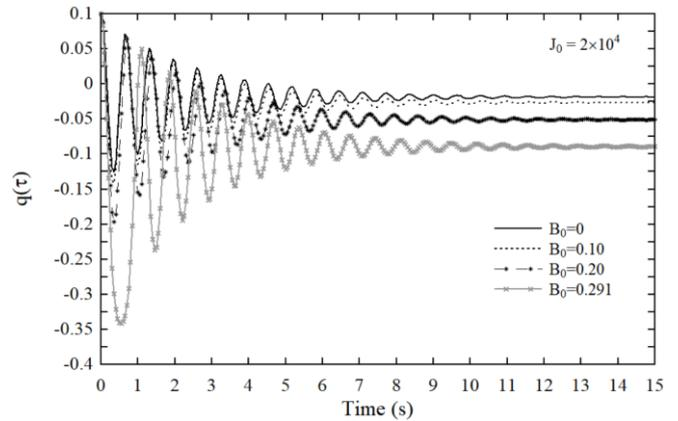
**Fig. 2. Effect of magnetic field intensity on the frequency response of a ferromagnetic plate with simple supports at both ends for current J0 = 2 A**
