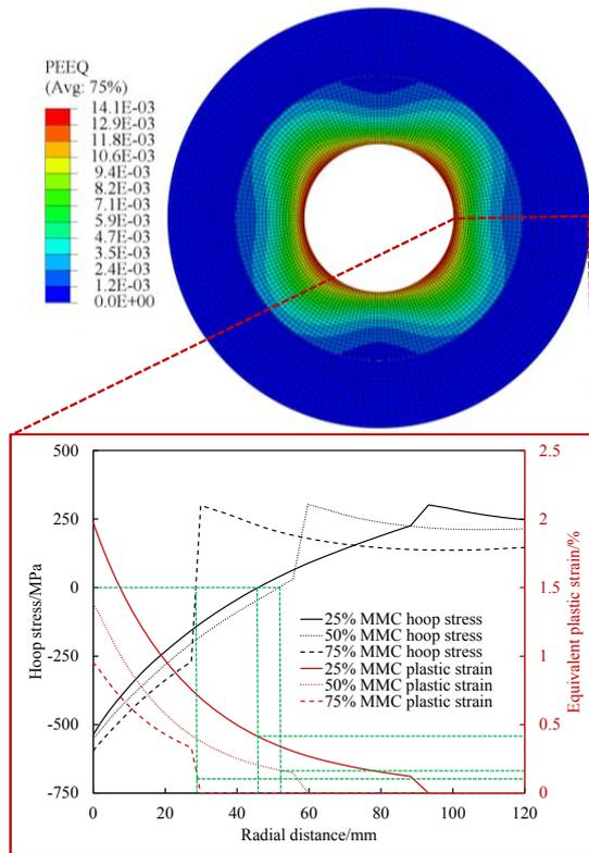
**Fig. 1. The hoop stress and the equivalent plastic strain along the radius in the cylinder with ST52 steel and metal-matrix composite materials**
