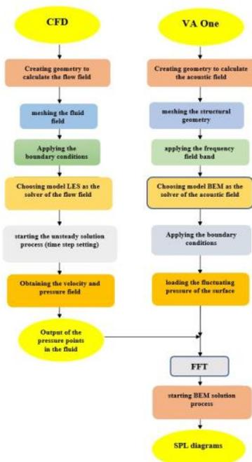
**Fig. 1. Schematic flowchart of hybrid CFD/BEM approach**
