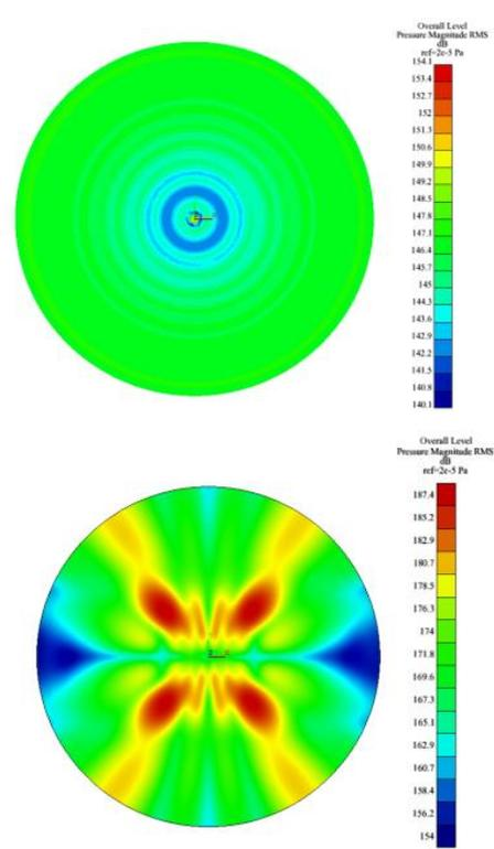
Fig. 5. a) Horizontal interface of the projectile without jet flow deflector, and b) horizontal interface of the projectile with a jet flow deflector.
