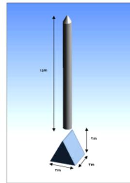
**Fig. 2. Dimensions of the projectile and jet flow deflector**
