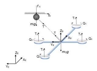
Fig. 2. Free diagram of the forces and torques for quadrotor-inverted pendulum system in a constrained motion
