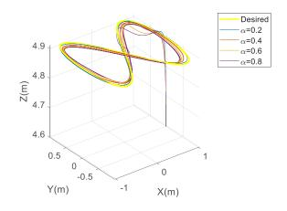
Fig. 4. Pendulum paths while tracking the desired trajectories vs the desired path.
