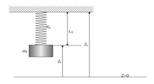
Fig. 3. Schematic of the model of the pendulum- ceiling interaction
