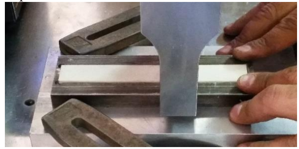
Fig. 1. Ultrasonic welding of the arms to make an ENF sample
