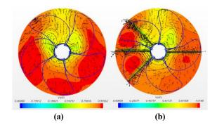
Fig. 3. Axial velocity (contour) and transverse velocity (vectors) in a section at a distance of 0.2D upstream of the propeller: (a) Without stator, (b) Four stators
