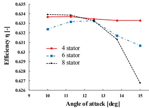
**Fig. 4. Comparison of the effect of stators on the efficiency of the propeller**
