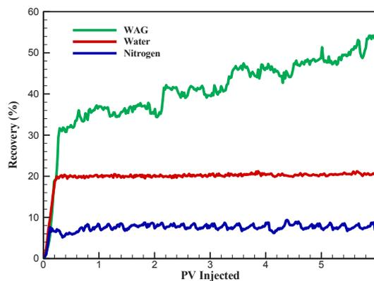
Fig. 2. Recovery vs PV injected in the S medium
