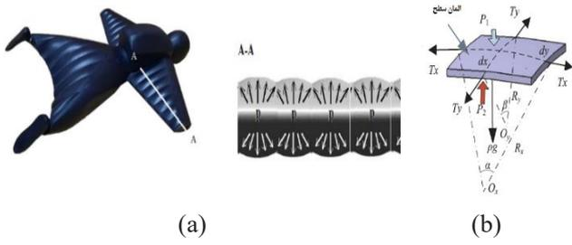
Fig. 1. pressure distribution inside of a wingsuit
