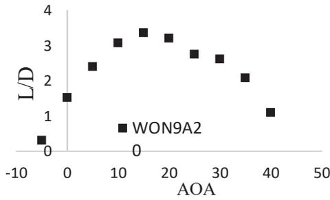
Fig. 3. Performance diagram (L/D) at Re= 1.5×10<sup>6</sup>
