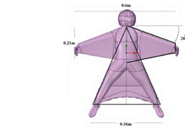
Fig. 2. The geometry of the wingsuit mode
