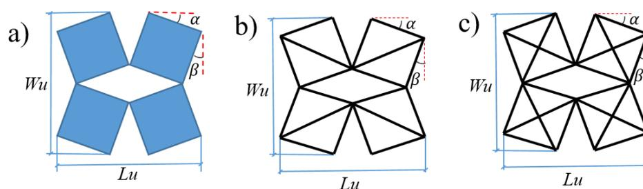
**Fig. 1. Creating auxetic structures inspired by structures with rotating blocks: a) a unit cell of the structure with rotating blocks, b) construction of a unit cell with similar behavior in two directions, c) a unit cell with completely identical properties in two directions.**
