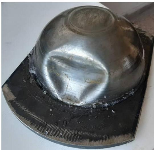
Fig. 2. final collapsed vessel
