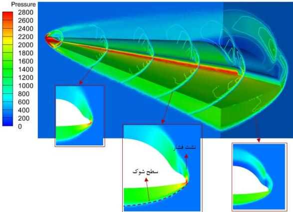
**Fig. 4. Pressure distribution around the HTV2 reference model**
