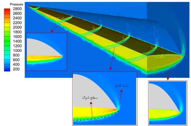
**Fig. 3. Pressure distribution around the superior designed configuration**
