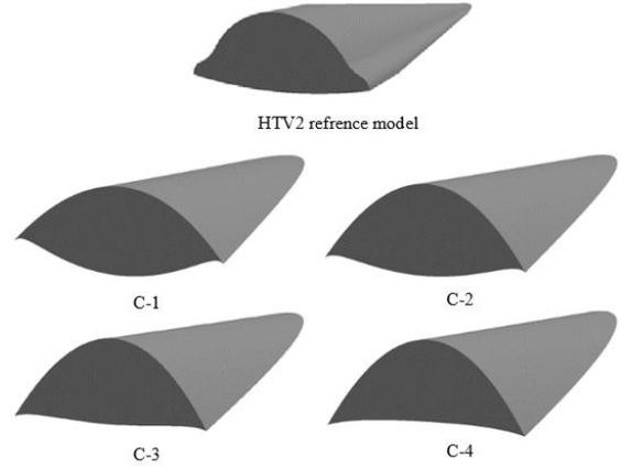
**Fig. 2. The HTV2 glide vehicle and the four designed configurations**
