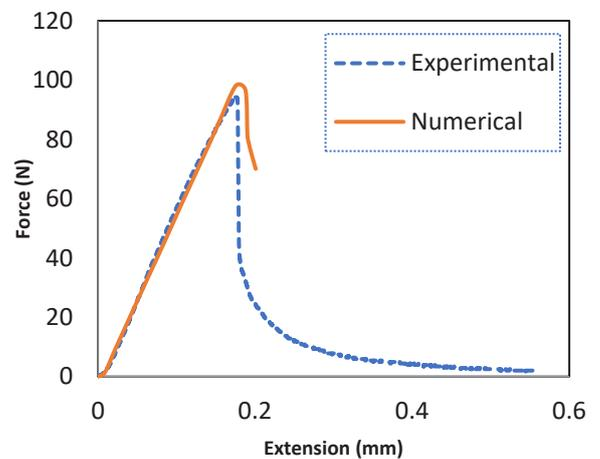
**Fig. 4. Numerical and experimental comparison diagram of perforated beam**
