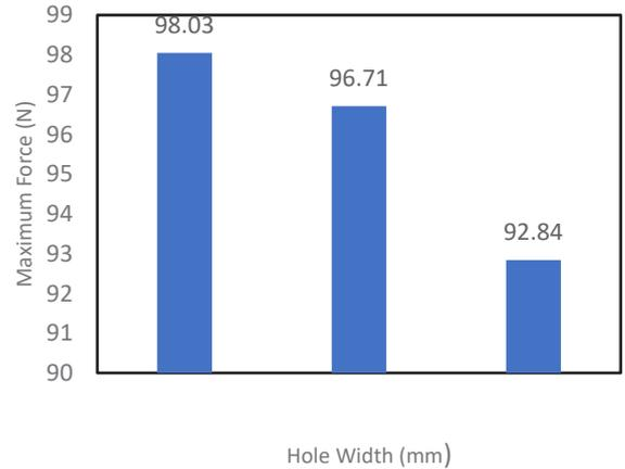
**Fig.3. The diagram of the maximum force obtained from the numerical analysis of the hole with a width of 2 mm and different lengths.**
