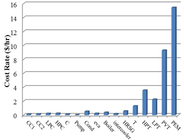
Fig. 3. The cost rate of different components of the system
