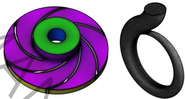
Figure 2. The grid generated for the impeller and volute
