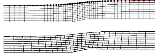
**Figure 1. Comparison of the final position of the free-surface, up) Default solver (black dots) and developed solver (red line), deown) Muzafarija and Peric [1]**
