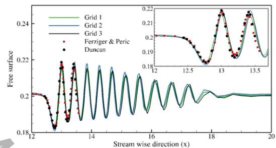
**Figure 2. Comparison of results for three grids with different resolutions and also comparison of free-surface waves with numerical and experimental results of [9]**
