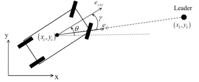
**Fig. 2. The vehicle direction relative to the direction of the leader's relative position.**
