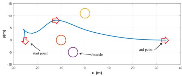
**Fig. 3. The trajectory of the autonomous vehicle moving among the multiple obstacles.**
