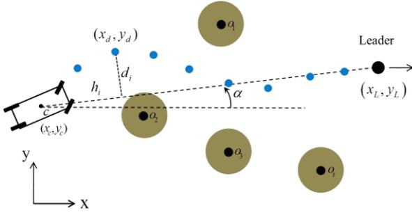
**Fig. 1. Optimal trajectory for leader following and obstacle avoidance.**
