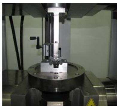
Fig.1. Fracture mechanics specimens used in this research, (a) geometry and design dimensions of 3PB samples, (b) photograph of test samples before fracture tests. The test specimens were machined in TL orientation (T is transverse loading direction and L is longitudinal crack
