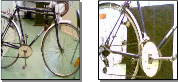
Fig3: a prototype bicycle which is made based on the optimal design sprocket wheel
