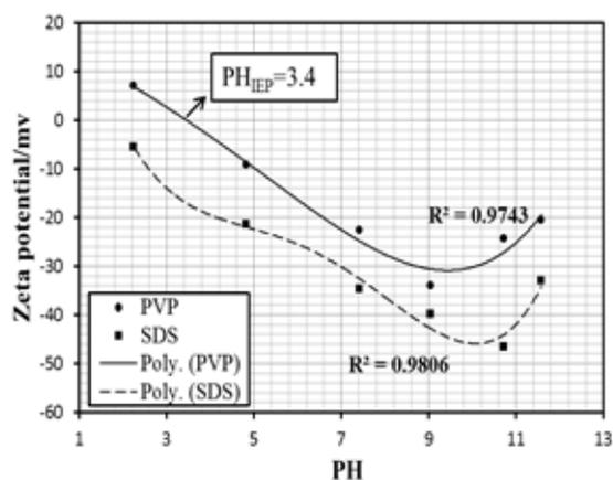
Figure 1. Effect of ph on zeta potential of CuO/deionized water nanofluid with SDS and PVP surfactants. concentration of cuo is 0.1 % (mass fraction)
