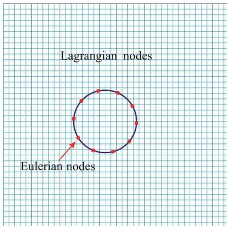
Fig.1. Schematic of immersed boundary method
