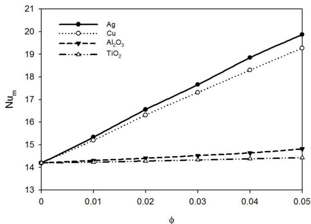
Figure 4. Variation of average Nusselt number with nanoparticles volume fraction for various types of nanoparticles ( $Ri=0.1$ )
