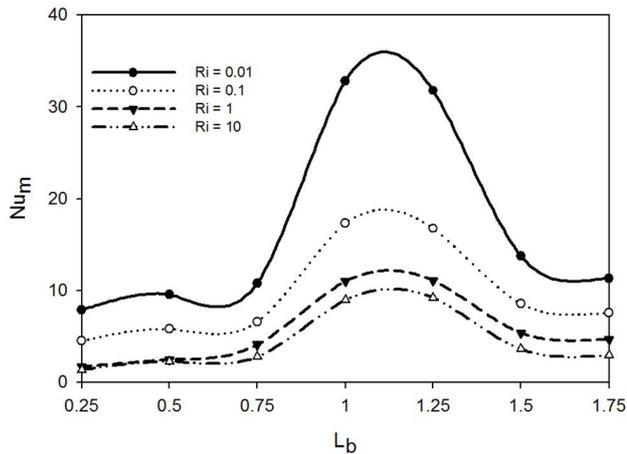
Figure 3. Variation of average Nusselt number with baffle location at various Richardson numbers (Cu-Water,  $\phi=0.03$ )
