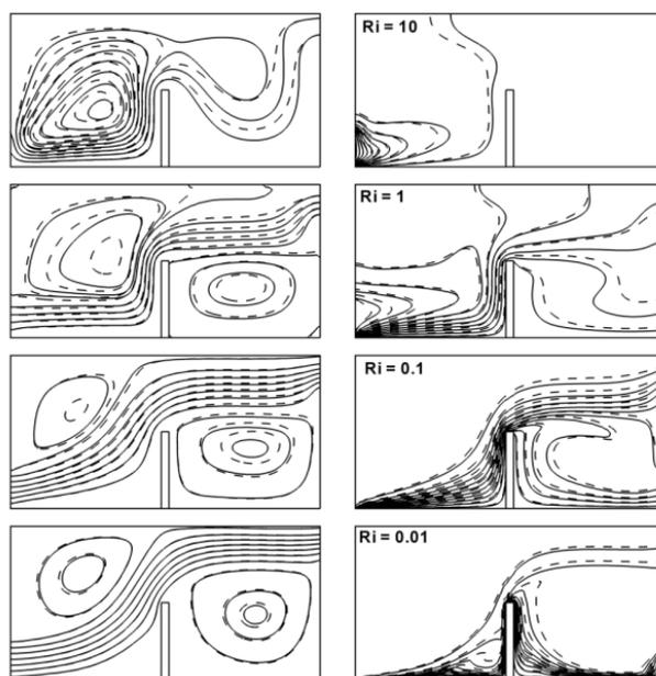
Figure 2. Streamlines (left) and isothermal lines (right) for different Richardson numbers (dash line: nanofluid( $\phi=0.03$ ) and filled line: water) ( $L_b=1$ )
