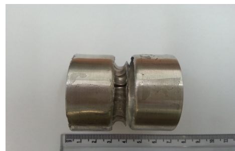
Figure 4. The final formed tube in the experimental test with 6200V, 0.6 mm thickness and 0.1mm clearance
