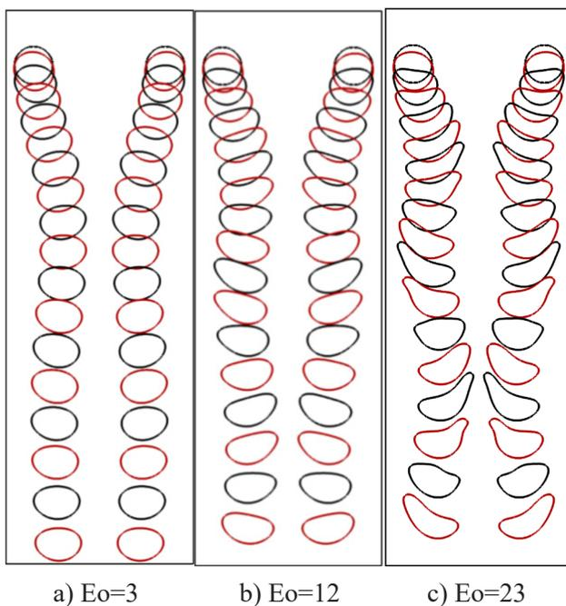
**Figure 1. Falling two adjacent droplets by different initial lateral positions from near the side walls ( $Oh=0.072$ ,  $t_0^*=0$ ,  $\Delta t^*=1$ )**
