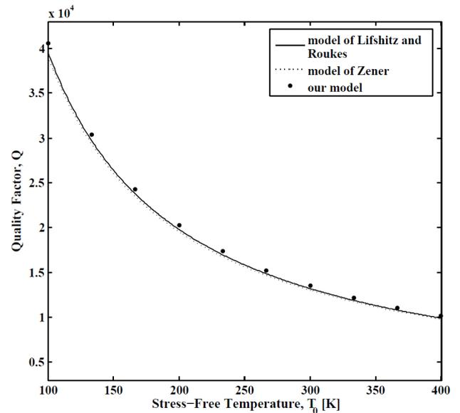
**Figure 2.** Comparison of the quality factors,  $Q$ , obtained using our model to those of Lifshitz and Roukes [3] and Zener [1,2] for various values of the stress-free temperature  $T_0$ .
