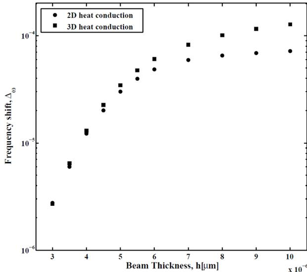
**Figure 1.** Comparison of frequency shifts computed using 3D theory of frequency shifts with the 2D exact results of Prabhakar et al [4].
