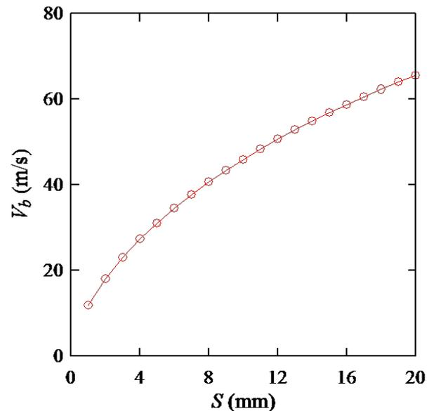
**Figure 2. Ballistic limit versus cell size of aluminum-honeycomb sandwich panel**
