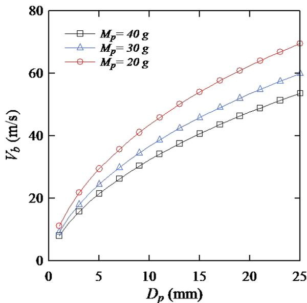
**Figure 1. Ballistic limit vs. ( $D_p$ ) for different projectile masses, at constant sandwich panel size and projectile density**
