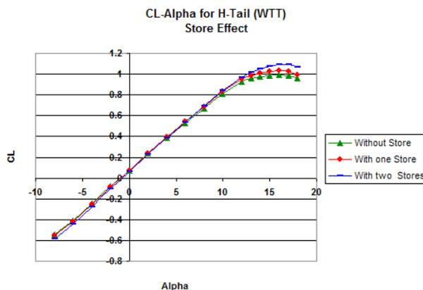
Figure 2.  $C_L - \alpha$  with and without external tank
