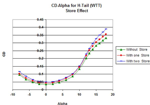
Figure 3.  $C_D - \alpha$  with and without external tank
