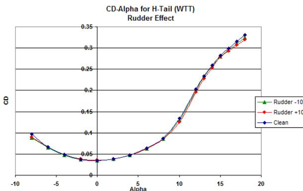
Figure 5.  $C_D - \alpha$  with variable rudder angle
