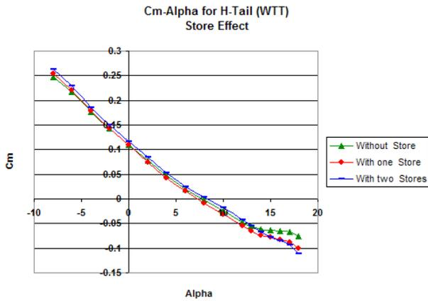
Figure 4.  $C_m - \alpha$  with and without external tank
