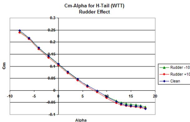
Figure 6.  $C_m - \alpha$  with variable rudder angle
