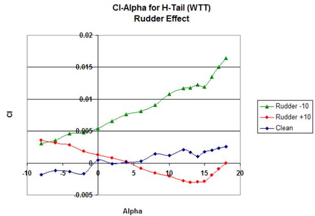
Figure 7.  $C_l - \alpha$  with variable rudder angle
