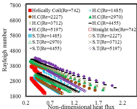
Figure 3. Rayleigh number as non-dimensional heat flux
